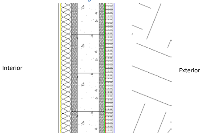
Figure 3 – The Enclosure Foundation Assembly (R20 eff. or R35 eff. with option stud bay insulation)
